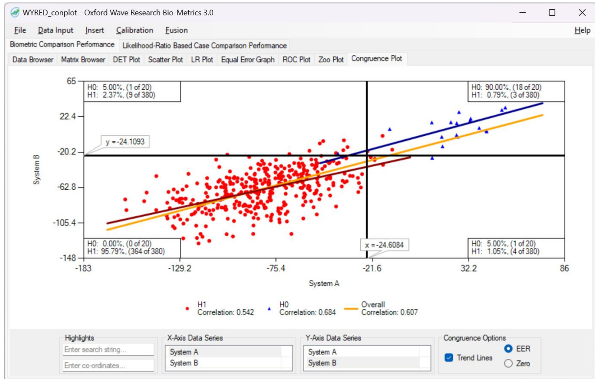
Figure 1: A congruence plot within Bio-Metrics software showing the scores output by two speaker recognition systems: System A (x-axis) and System B (y-axis). Same-speaker (H0) scores are indicated by blue triangles, and different-speaker (H1) scores by red circles. In this example, the axes are divided based on the EER score threshold. The H0 and H1 occupancy is indicated in each quadrant.
